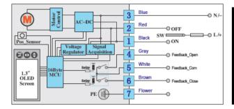
AVA electric actuators are supplied with a flying lead, models 20 only. Models 60 and above have terminal strip. No need to remove actuator housing to wire. See specific actuator model for exact wiring details.
