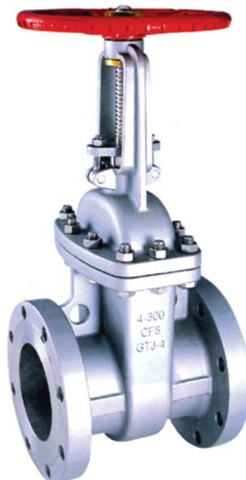
Stainless Steel Body, Bonnet & Wedge, Rising Stem, Handwheel Operated
