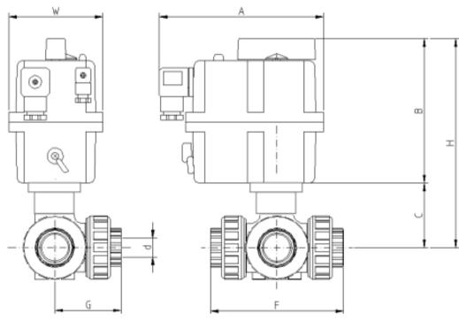
Note that dimensions and above image show a generic PVC valve and the J+J actuator. For exact dimensions for your specific requirement, call the office for confirmation of dimensions. The following codes are based upon standard 3 way valve with imperial plain ends, PTFE/EPDM.
